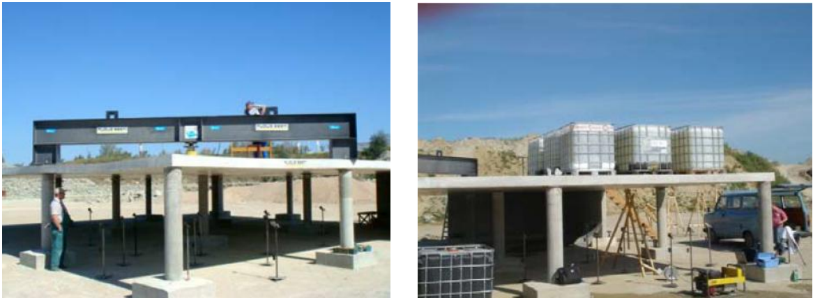
Figure 3.19: Hydraulic loading at centre span to the left and loading with “service load” to the right. (Destrée, 2008).
