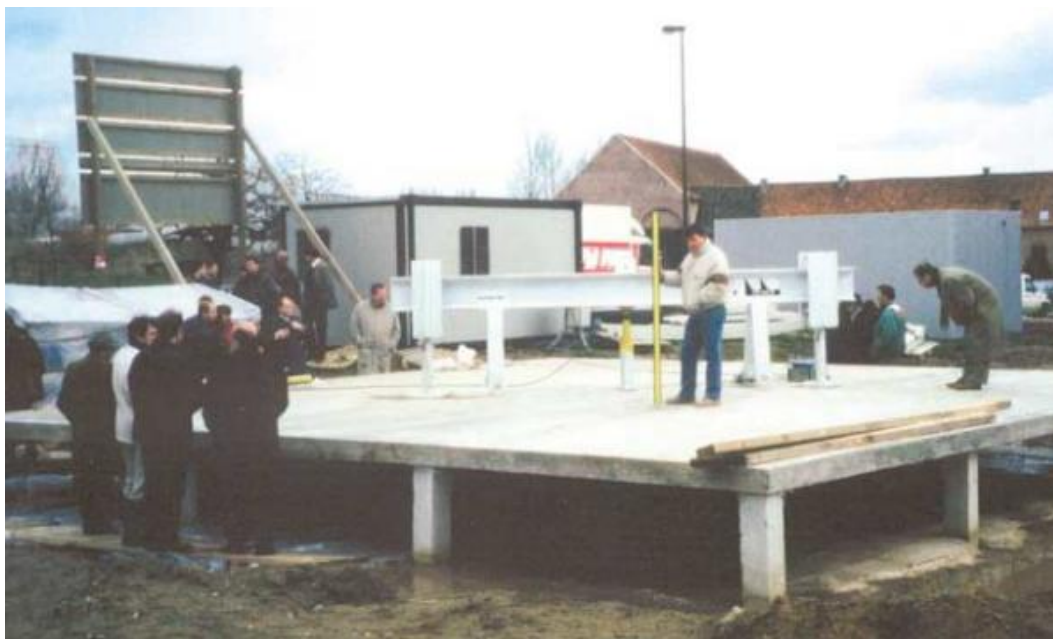
Figure 3.11: Full-scale loading with a centre load applied with a loading frame. (Destrée, 2001)
