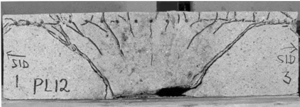
Figure 3.1: Punching shear cracks in a circular RC plate punching test, from (Hallgren, 1998)
