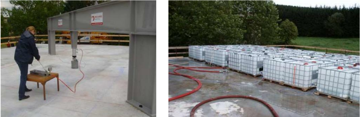
Figure 3.15: Hydraulic loading at centre span to the left and loading with “service load” to the right. (Destrée, 2008).
