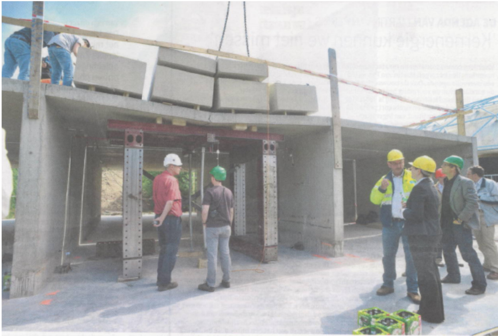
Figure 3.23: The gravitational loading was 1.0 \text{ ton/m}^2 / w_{\text{direct}} = 3 \text{ mm} , w_{1\text{day}} = 10 \text{ mm} and at 1.3 \text{ ton/m}^2 the failure was sudden. (Tissink, 2011a).
